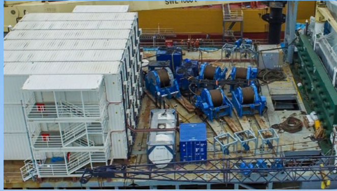
ADDITIONAL MOORING WINCHES AND LIVING QUARTER
